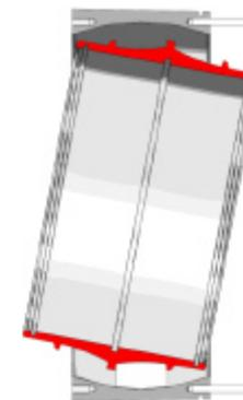
4. Rotate the inner race and 4-5 rollers so the opposite side of the roller track that has the first 4-5 rollers in it just exposed at the upper edge and a roller can be placed in the track.
